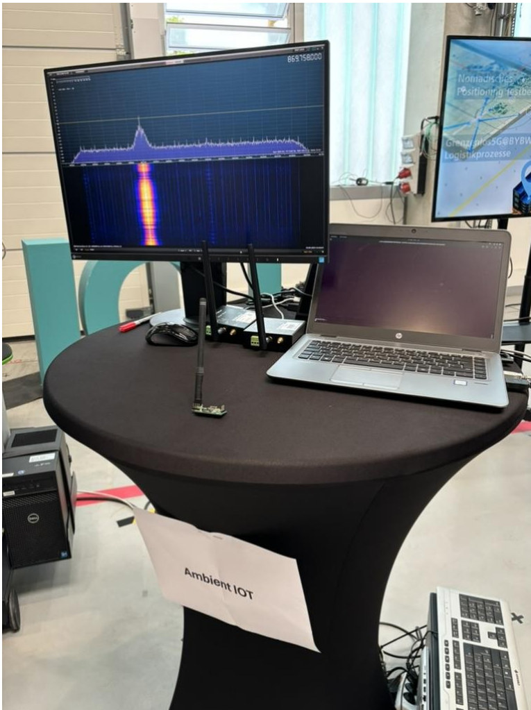
Figure 12: Experimental device for Ambient IoT utilising 'back scattering'. Source: Fraunhofer IIS, 5G Connect Advanced (19 September 2024).
